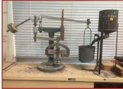
Figure 1. Three-point flexural strength test
