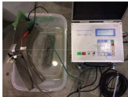
Figure 3. Mortar resistance measurement
